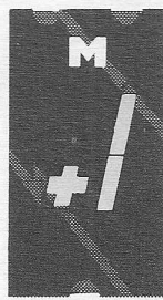
MAN 83 Common Anode; Overflow ( \pm 1 )
